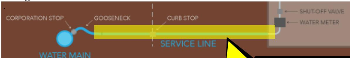
To achieve LSLR requirements, you must replace all galvanized service lines that **is or was** downstream of lead piping.
