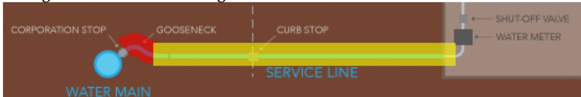
To achieve LSLR requirements, you must replace the lead gooseneck and all galvanized downstream.
