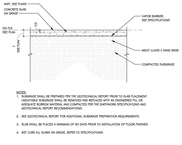
TYPICAL SOG CONSTRUCTION SCALE: NONE
