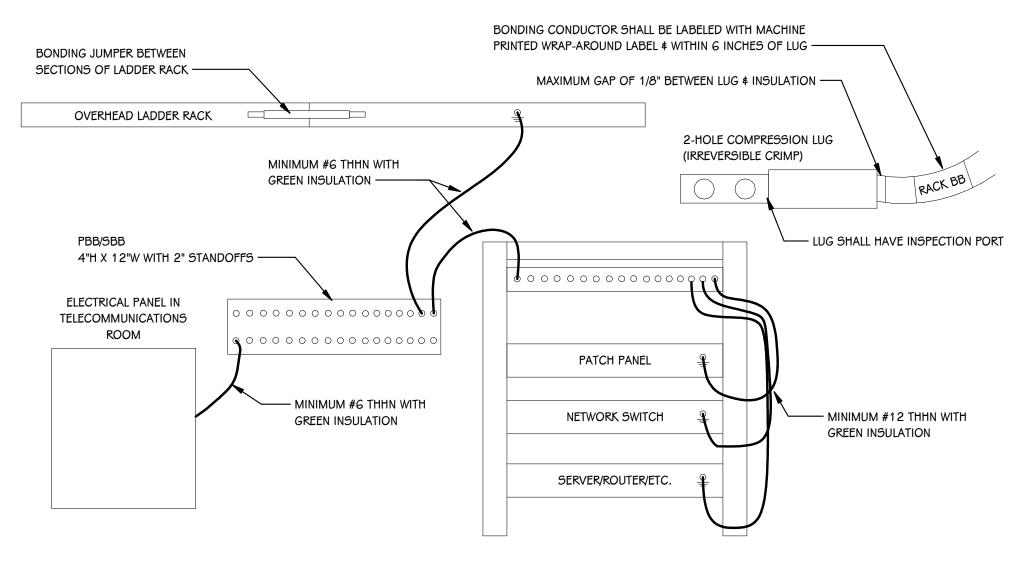
TELECOMMUNICATION ROOM BONDING DETAIL
