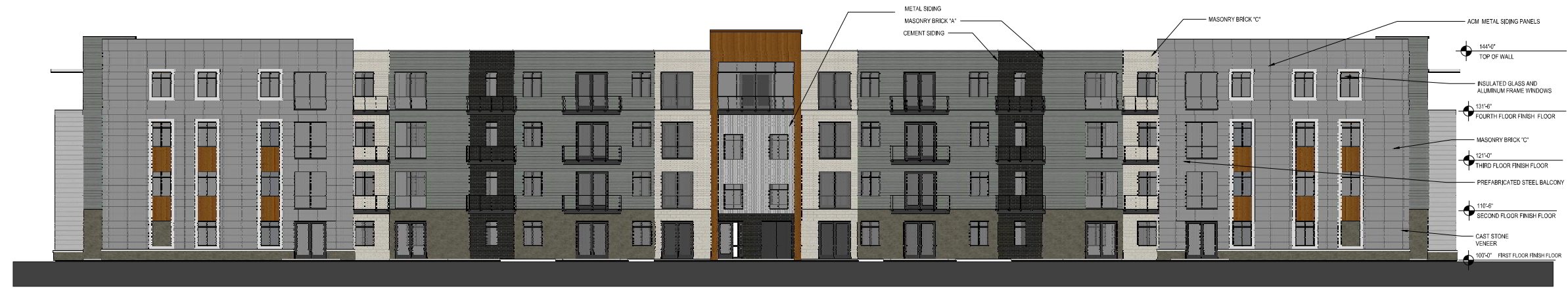
SOUTH ELEVATION - OPTION 01 3/32" = 1'-0" COLORS / FINISHES TO BE SELECTED FROM MANUFACTURER'S STANDARD COLORS AND FINISHES
