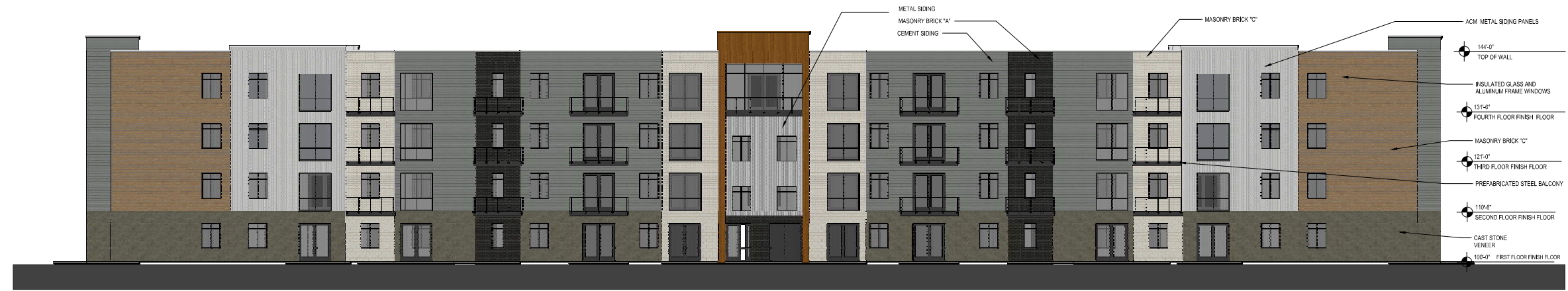
SOUTH ELEVATION - BUILDING A 3/32" = 1'-0" COLORS / FINISHES TO BE SELECTED FROM MANUFACTURERS STANDARD COLORS AND FINISHES
