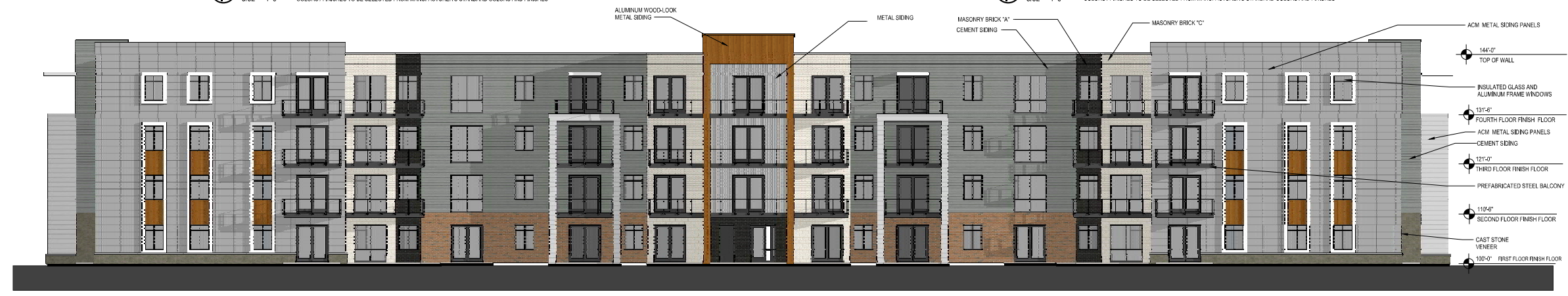
NORTH ELEVATION - OPTION 01 3/32" = 1'-0" COLORS / FINISHES TO BE SELECTED FROM MANUFACTURER'S STANDARD COLORS AND FINISHES
