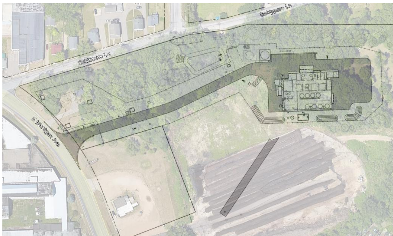
Figure 3-4. Treatment Plant Footprint at PS 5
