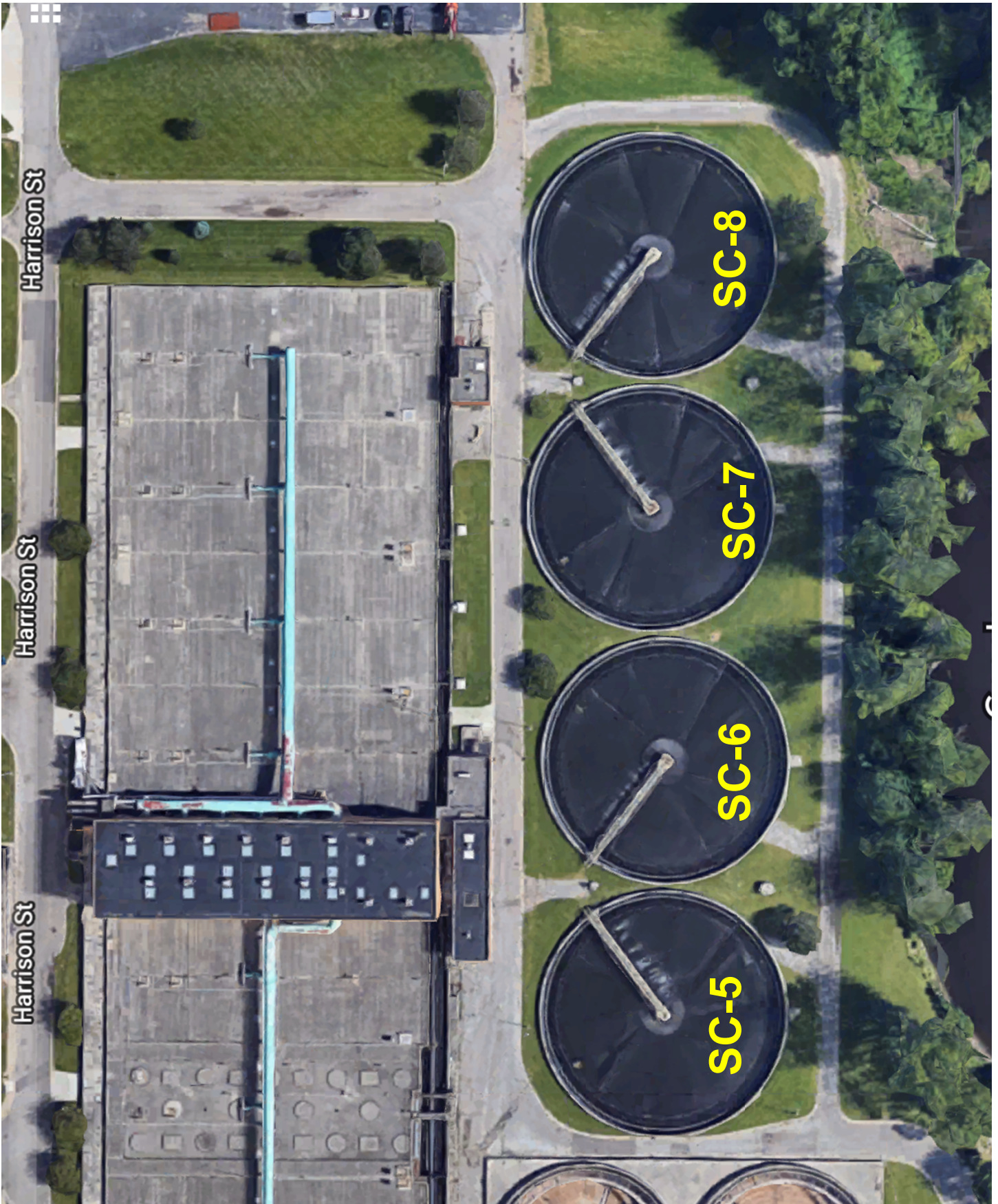
Secondary Clarifier Layout
