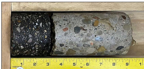
**Core picture shows approximate thickness CORE LOG DCP 1 meter rod (standard).XLS ver. 2/7/14 - Sand DCP
