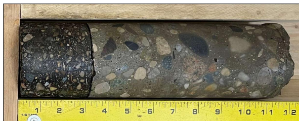
**Core picture shows approximate thickness CORE LOG DCP 1 meter rod (standard).XLS ver. 2/7/14-Sand DCP
