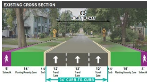
Figure 8-2: Existing Cross Section of Douglas Avenue
