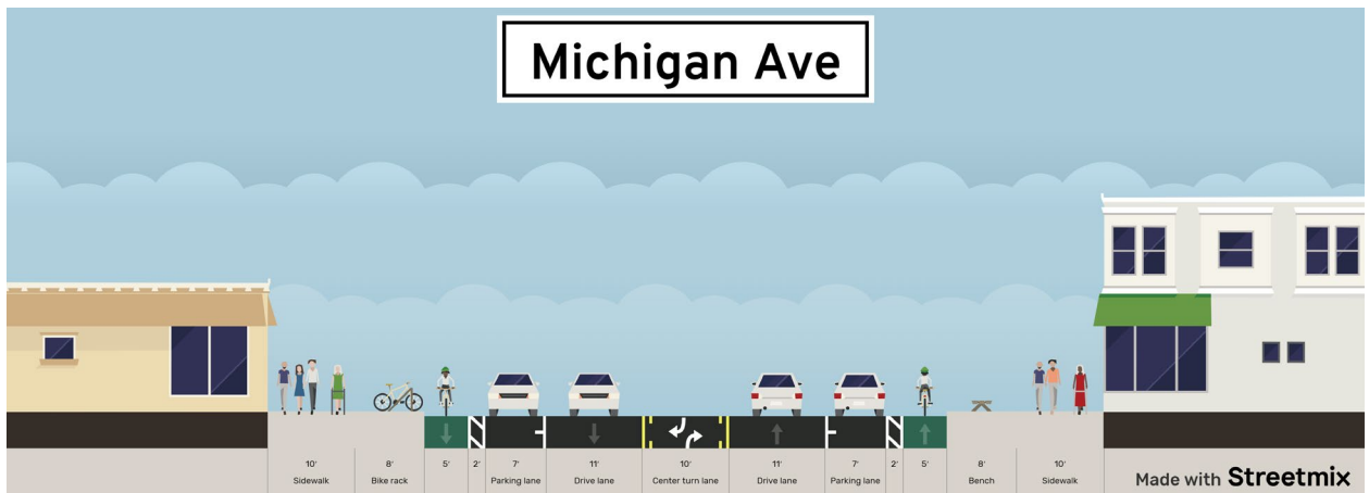
Figure 2-3: Proposed Cross Section for Michigan Avenue with Bike Lanes outside the Parking Lane
