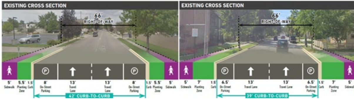
Figure 5-2: Commercial Lovell Street
