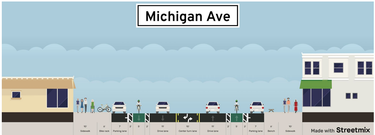
Figure 2-2: Proposed Cross Section for Michigan Avenue with Bike Lanes inside the Parking Lane
