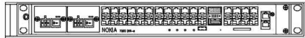
NOKIA - CSR IXRE V2 ROUTER WEIGHT: 11.2 LBS SIZE (HxWxD): 1.25 x 17.25 x 10.0 IN.
